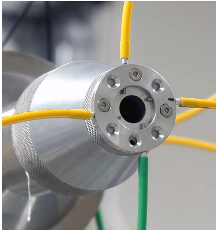
Figure 1: Closeup of the test nozzle with the tangential blowing injectors.
