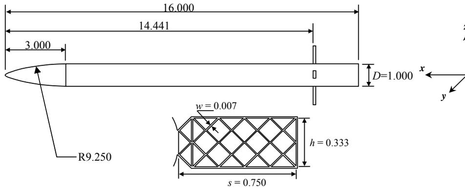
Figure 1. Schematic of the ogive cylinder with grid fin configuration (adapted from Ref. [4]).
