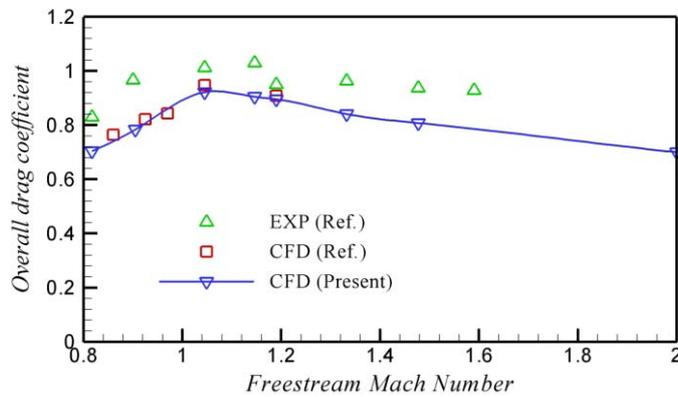
Figure 5. Comparison of the drag force coefficient between present CFD results and given data by Ref. [4]
