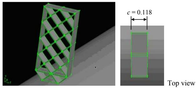
Figure 2. Schematic of the baseline grid fin configuration
