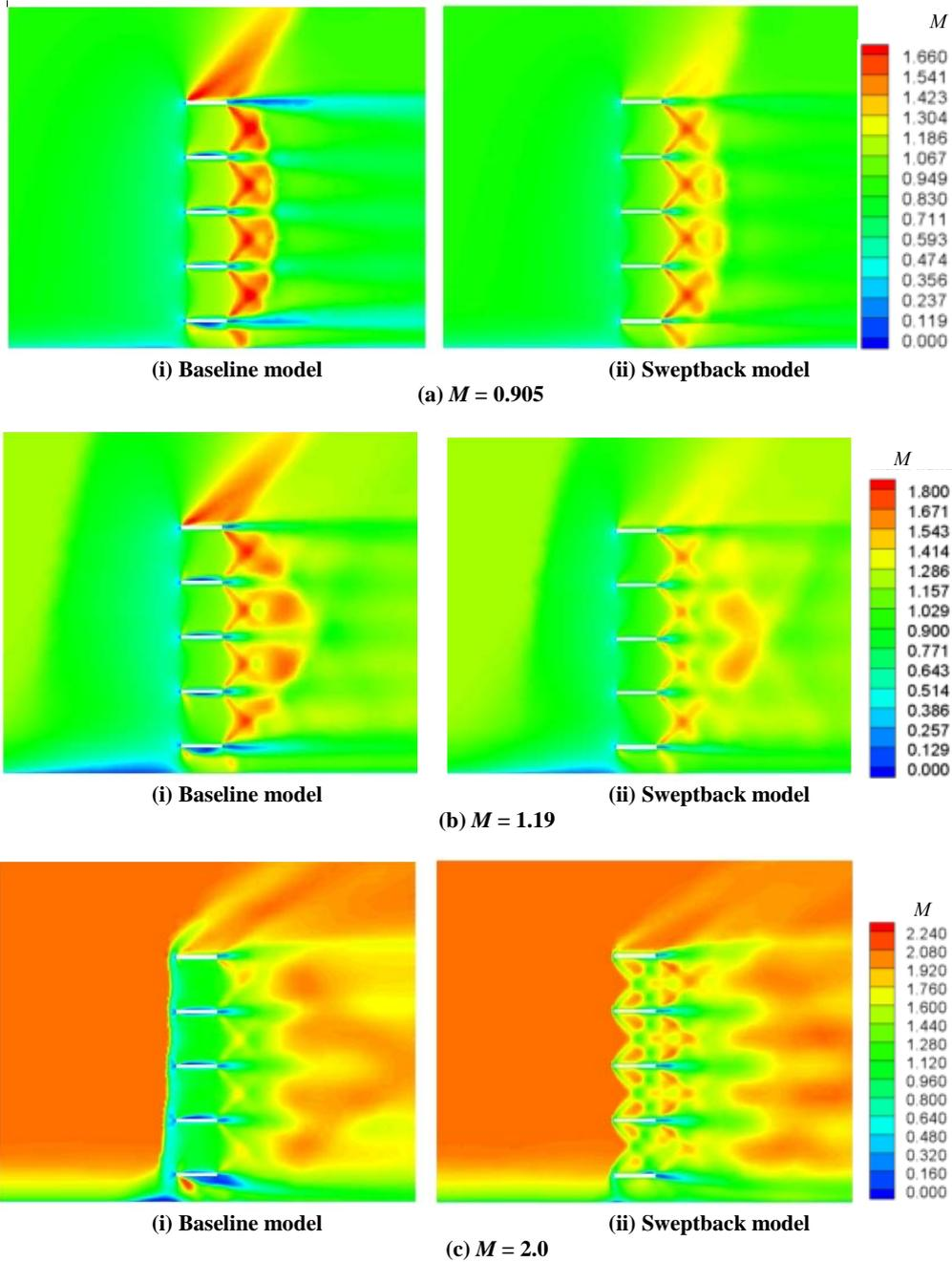
Figure 6 Mach number contours for the baseline and sweptback models at symmetry surface for freestream  $M=0.905$ ,  $1.19$ , and  $2$
