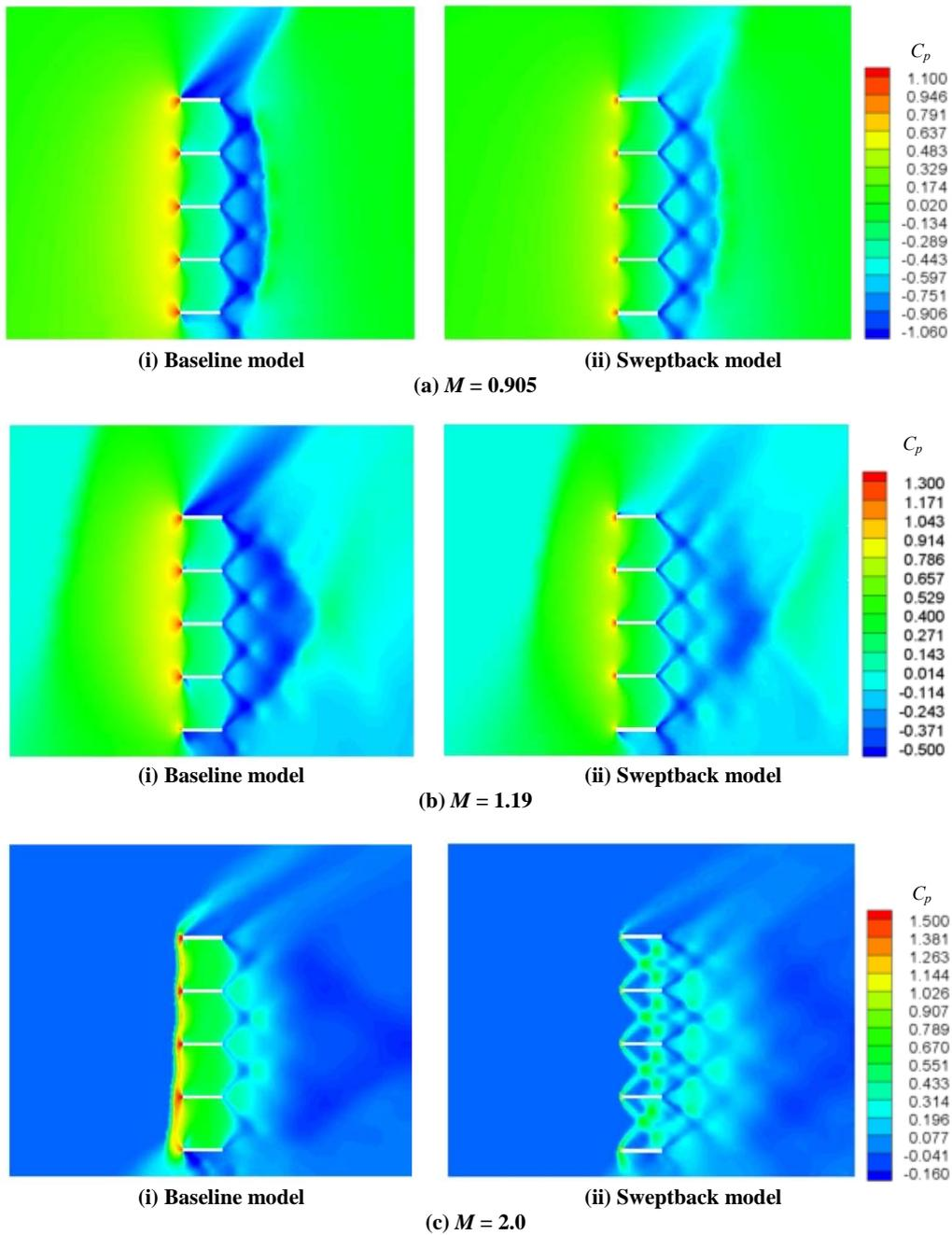
Figure 7 Pressure coefficient contours for the baseline and sweptback models at symmetry surface for freestream  $M=0.905$ ,  $1.19$ , and  $2$
