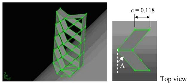
Figure 3. Schematic of the sweptback grid fin configuration
