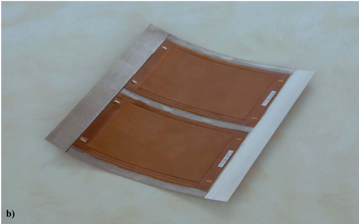
**Figure 2. Airfoil model for testing: a) assembled model; b) inner side of the upper skin with MFC patches.**
