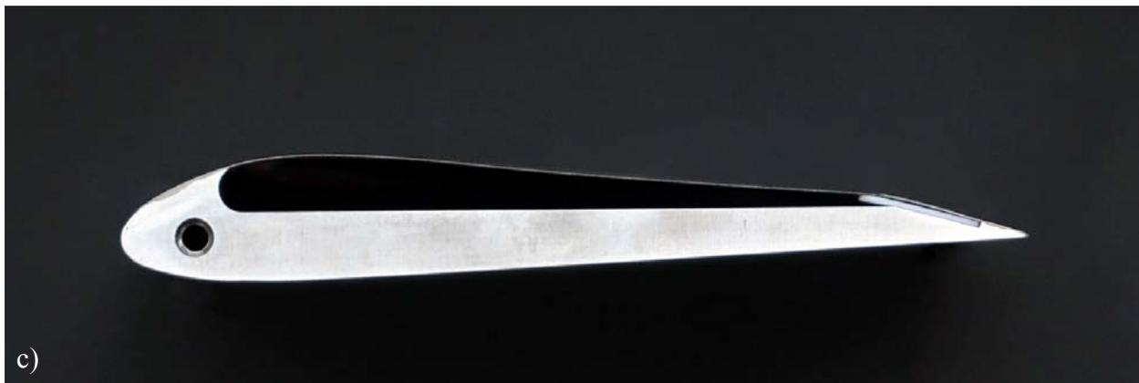
**Figure 5. Lateral view of the airfoil model: a) without actuation (shape similar to the NACA 4415 airfoil); b) with actuation at -500 V (3 mm maximum outward displacement); c) with actuation at 1500 V (5 mm maximum inward displacement).**
