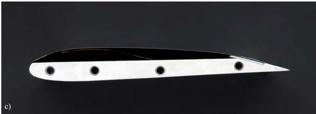
**Figure 5. Lateral view of the airfoil model: a) with actuation at -500 V (shape similar to a NACA 4415 airfoil); b) without actuation (about 1.4 mm inward displacement); c) with actuation at 1000 V (about 3.1 mm maximum inward displacement).**
