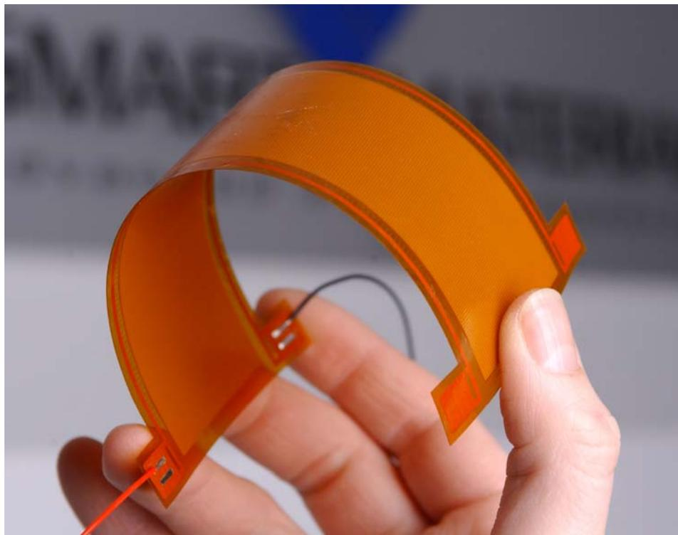
**Figure 1. Macro fiber composite (MFC) actuator [image courtesy of Smart Material Corp.].**
