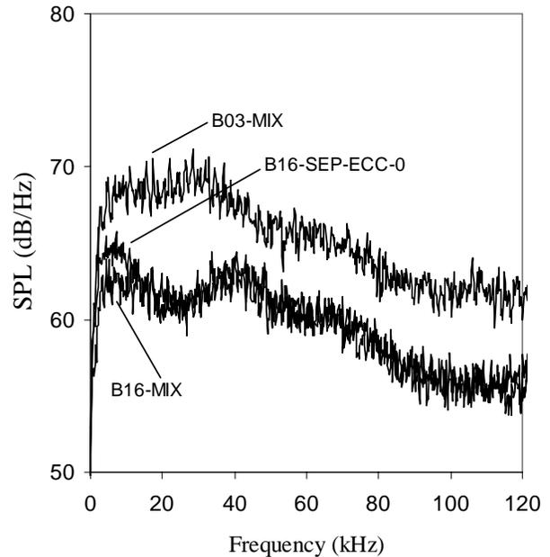
Fig.8 Far-field spectra at  $\theta = 90^\circ$ : baseline engine (B03-MIX); modified mixed-flow engine (B16-MIX); and modified separate-flow engine with eccentric exhaust, measured at zero azimuth angle (B16-SEP-ECC-0).
