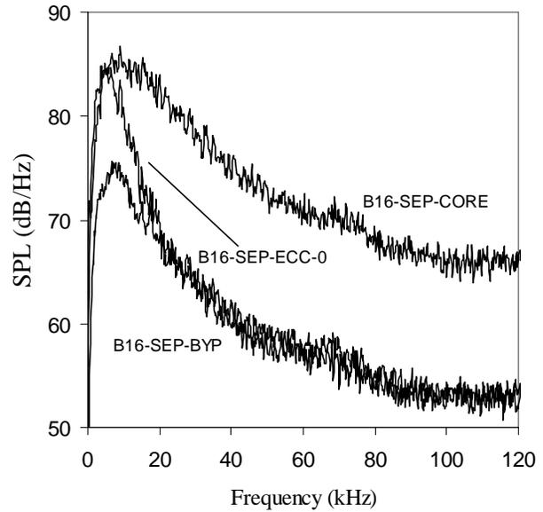
Fig.7 Far-field spectra in the direction of peak emission ( $\theta = 40^\circ$  for all spectra shown), not scaled to equal thrust: core stream only of modified separate-flow engine (B16-SEP-CORE); eccentric bypass stream only of modified separate-flow engine (B16-SEP-BYP); and modified separate-flow engine with eccentric exhaust measured at zero azimuth angle (B16-SEP-ECC-0).
