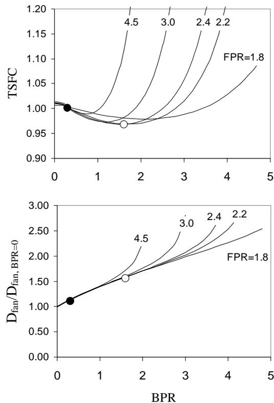
**Fig.1 Thrust specific fuel consumption and fan diameter, normalized by turbojet value, versus bypass ratio and fan pressure ratio for Mach 1.6 cruise. Solid and open symbols indicate the baseline and modified engines of this study, respectively.**
