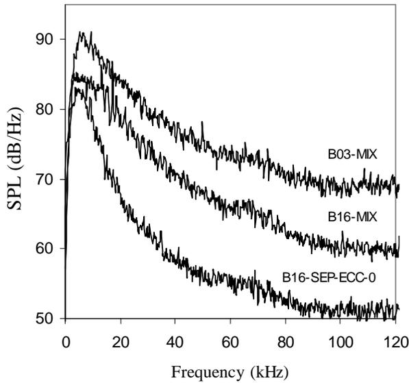
Fig.5 Far-field spectra in the direction of peak emission and scaled to equal thrust: baseline engine (B03-MIX,  $\theta = 40^\circ$ ); modified mixed-flow engine (B16-MIX,  $\theta = 25^\circ$ ); and modified separate-flow engine with eccentric exhaust, measured at zero azimuth angle (B16-SEP-ECC-0,  $\theta = 40^\circ$ ).
