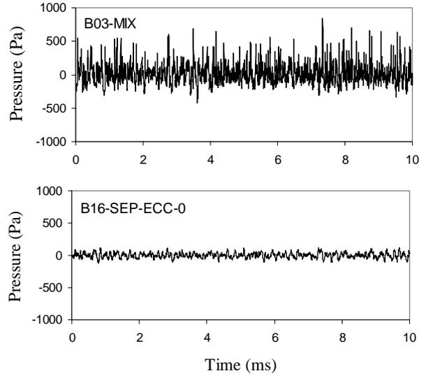
Fig.10 Microphone time traces in the direction of peak emission for baseline engine (B03-MIX) and modified separate-flow engine with eccentric exhaust, measured at zero azimuth angle (B16-SEP-ECC-0).
