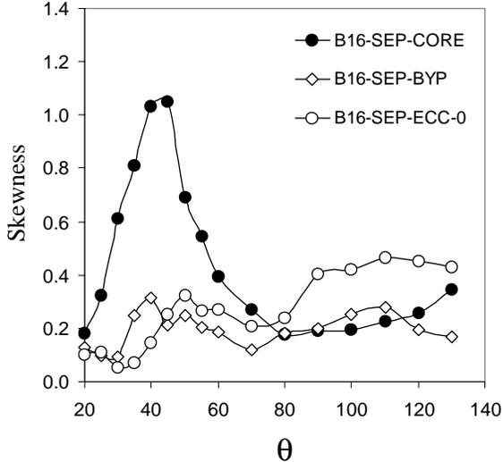
**Fig.12 Directivity of normalized skewness for: core stream only of modified separate-flow engine (B16-SEP-CORE); eccentric bypass stream only of modified separate-flow engine (B16-SEP-BYP); and modified separate-flow engine with eccentric exhaust measured at zero azimuth angle (B16-SEP-ECC-0).**
