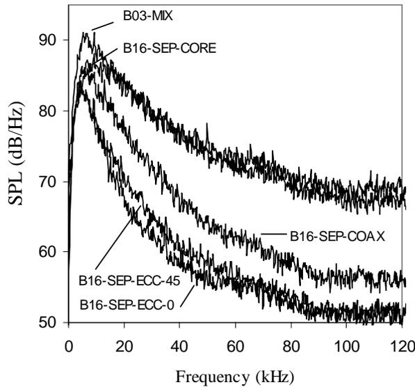
Fig.6 Far-field spectra in the direction of peak emission ( $\theta = 40^\circ$  for all spectra shown) and scaled to equal thrust: baseline engine (B03-MIX); core stream only of modified separate-flow engine (B16-SEP-CORE); modified separate-flow engine with coaxial exhaust (B16-SEP-COAX); and modified separate-flow engines with eccentric exhaust, measured at zero and  $45^\circ$  azimuth angles (B16-SEP-ECC-0, B16-SEP-ECC-45).
