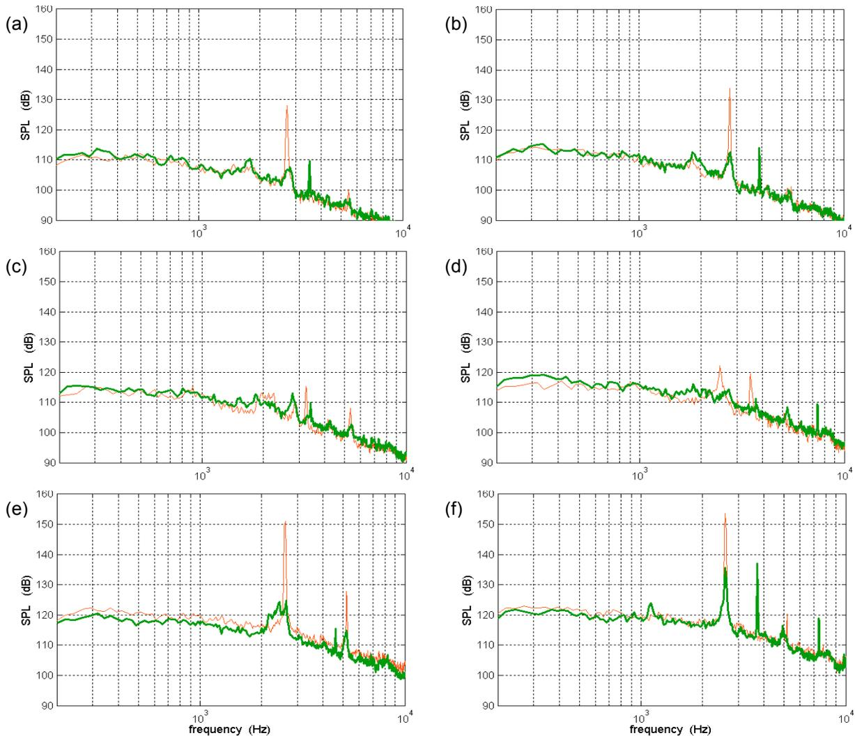
Figure 12: Noise spectra of the unforced cavity flow (thin line) and of the same flow controlled with optimal frequency forcing at  $4 V_{rms}$  (thick line) at selected Mach numbers: (a)  $M = 0.26$ ; (b)  $M = 0.29$ ; (c)  $M = 0.32$ ; (d)  $M = 0.37$ ; (e)  $M = 0.43$ ; (f)  $M = 0.46$ .
