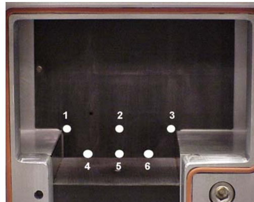
Figure 2. Location and numbering of Kulite pressure transducers in the cavity flow.
