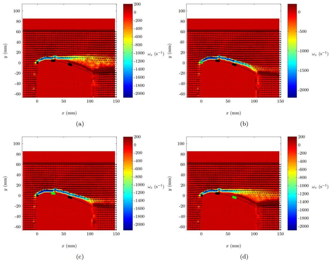
Fig. 3 Velocity vector and vorticity contour plots with the upper surface airfoil curvature and the actuators for an angle of attack of  $10^\circ$  and  $Re = 35000$ : (a): no actuation; (b): 1<sup>st</sup> actuator on (green rectangle); (c): 2<sup>nd</sup> actuator on (green rectangle); (d): 3<sup>rd</sup> actuator on (green rectangle).
