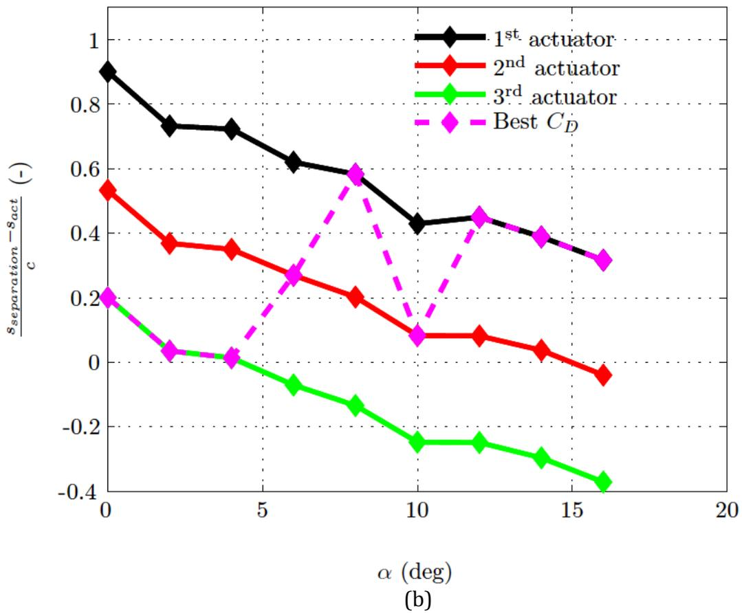
Fig. 4 Evolution of the non-dimensional curvilinear distances between the flow separation points and the actuator locations with the angle of attack for  $Re = 35000$ : (a): actuators associated with the best  $C_L$  underlined with a dotted blue line; (b): actuators associated with the best  $C_D$  underlined with a dotted magenta line.
